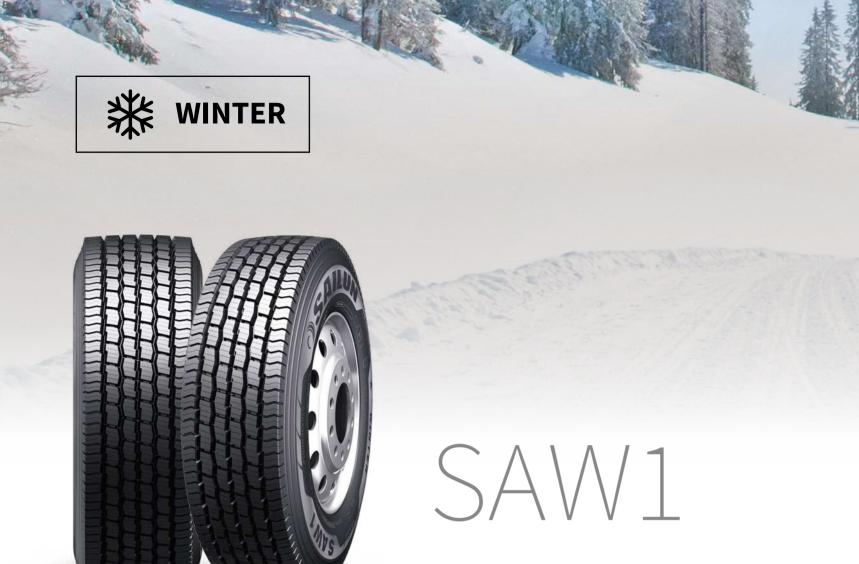
The new SAW1 is an all-position specialty winter tyre that improves handling on ice and snow. The wide tread width and five main grooves increase the tyre's contact area and improves grip. M+S and 3PMSF identification represent the tyre's excellent winter performance. Unique sipe pattern and open shoulder design effectively drain water.
