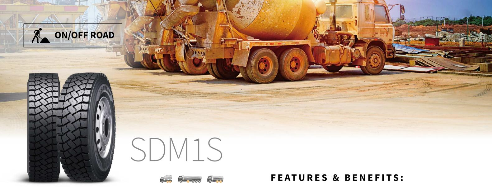
The SDM1S Tyre employs large blocks with deep grooves which have strong resistance to puncturing, chunking, and provide excellent traction. The groove design effectively reduces stone retention to improve casing protection and tread life. The tyre is especially useful on poor road conditions.
