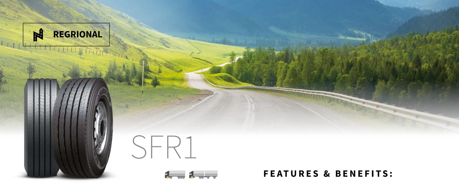
The SFR1 is a steer position tyre suitable for mid to long distance trucks and busses running on good roads. Tread compound formula improves scrub resistance. Unique shoulder design and deeper shoulder grooves help prevent abnormal tyre wear. Widened running surface provides better tread-to-ground contact area for improved handling.
